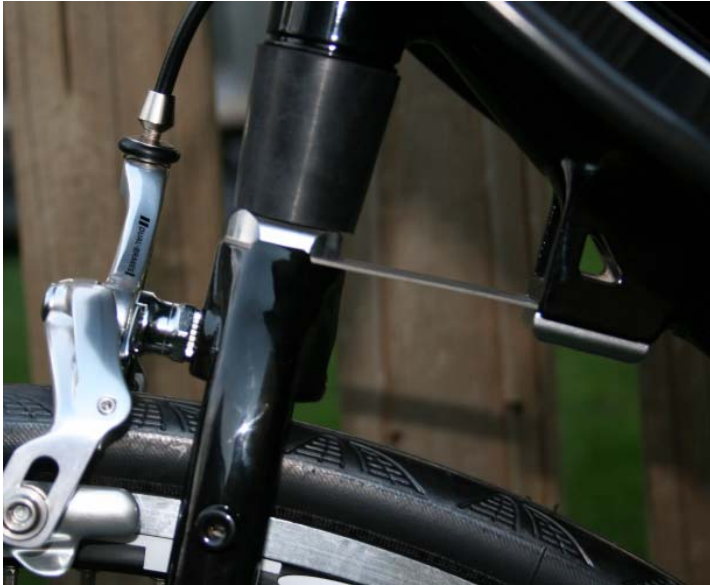
Titanium leaf spring and a progressive-rate elastomer
